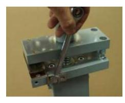
Mount the back paper stops with two M6x10 screws and washers on the paper punch. Use a 10mm wrench to fix the screws.
