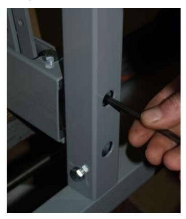
**3.** The foot pedal during the delivery fixed only with one screw. Loose this crew and set in the right position the pedal.
