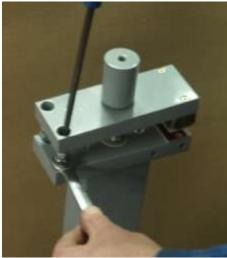
Release the female screw of the M8 setting screws at the back of the machine, set the parallelism and fix the screw again.
